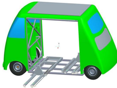
Figure 1. A representation of the FURBOT vehicle, with the load area and its fork lift system.
